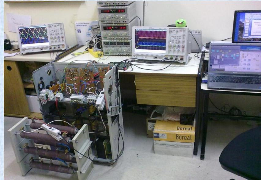
Multilevel Current Source inverter
